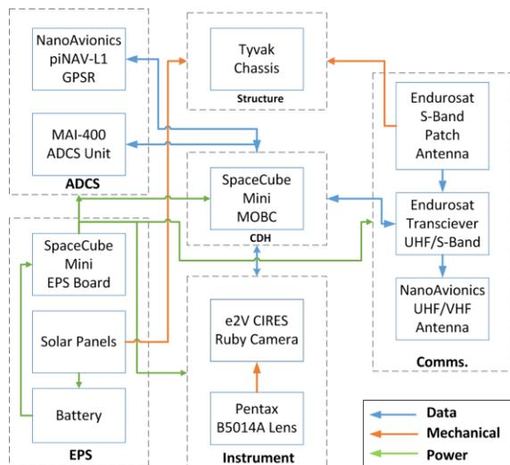
**Figure 6: System architecture for the Observer Satellite (OSat).**
