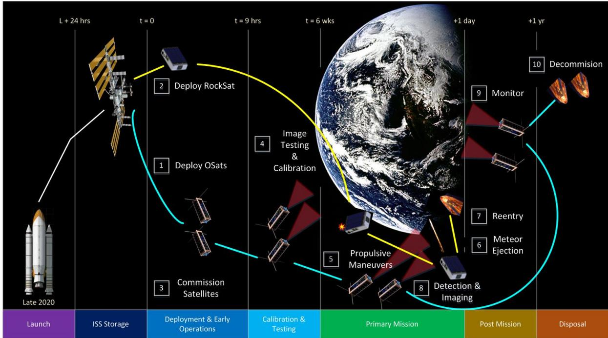
**Figure 3: Concept of Operations for the Space Weather and Meteor Impact Monitoring Network (SWIMNet).**
