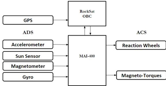
Figure 9: RockSat ADCS architecture
