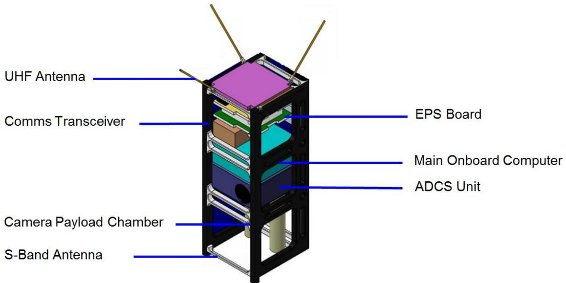
**Figure 4: Observer Satellite (OSat).**
