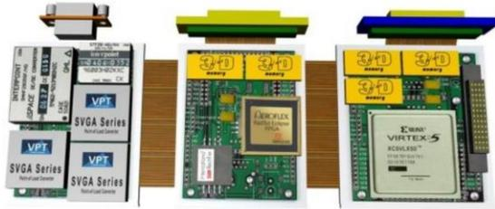
**Figure 19: SpaceCube MINI folded flat**
