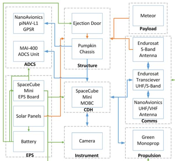
**Figure 7: System architecture for the Rock Satellite (RockSat).**
