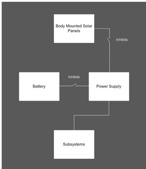
**Figure 18: Electrical Power Subsystem Architecture for OSat & RockSat.**
