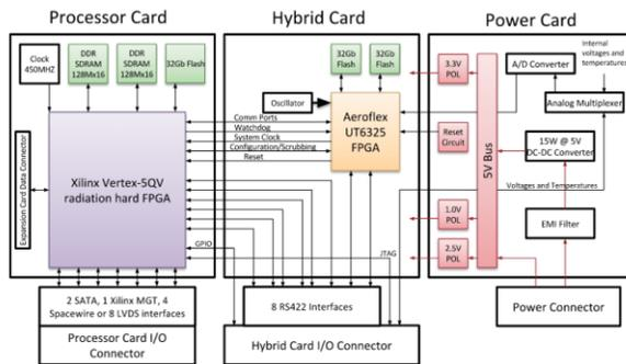
**Figure 20: SpaceCube Mini architecture**
