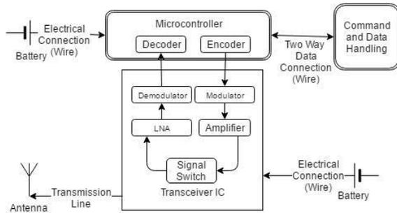
Figure 16: Communication system architecture
