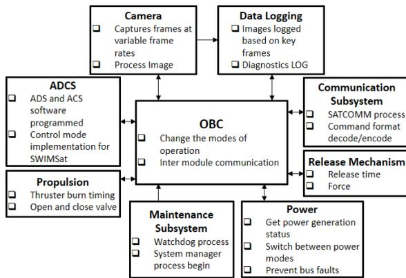
**Figure 22: RockSat Software architecture**
