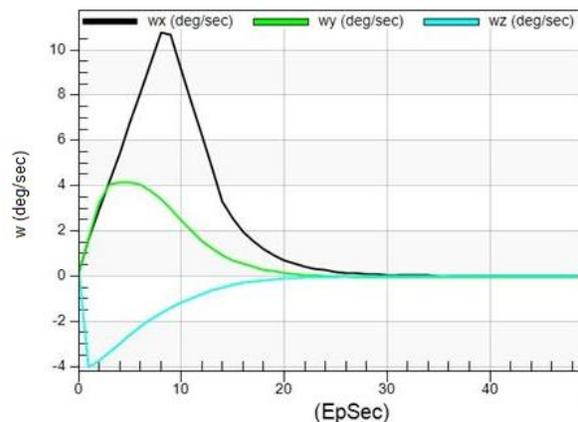
Figure 13: Communication pointing mode (angular velocity).
