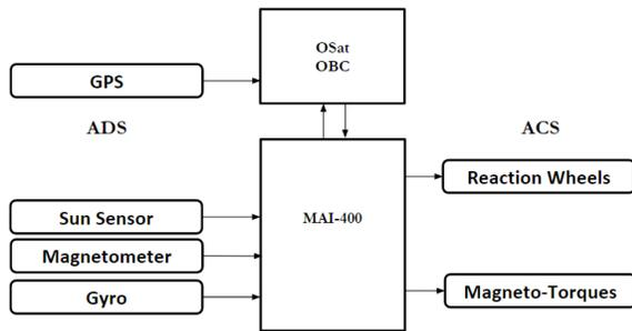
Figure 10: OSat ADCS architecture
