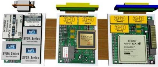
**Figure 19: SpaceCube MINI folded flat**
