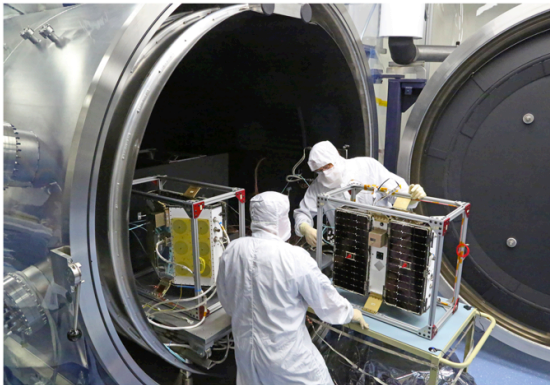
Figure 10: CYGNSS Entering Thermal Vacuum Testing
