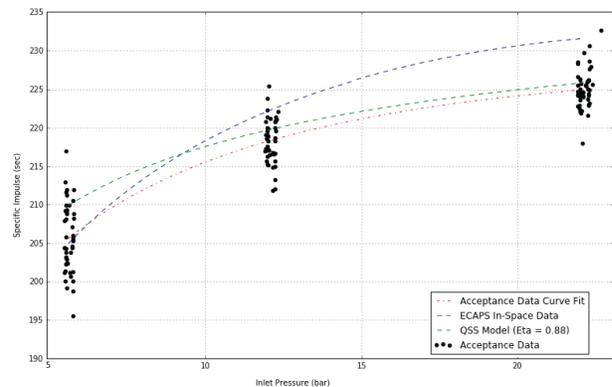
**Figure 8.** 100% Duty-Cycle Acceptance Test Results (Isp) for 1N HPGP thrusters integrated into SkySat propulsion systems
