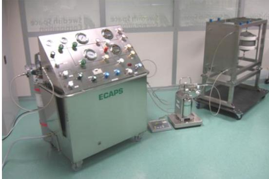
**Figure 12.** LMP-103 Fueling Set-up
