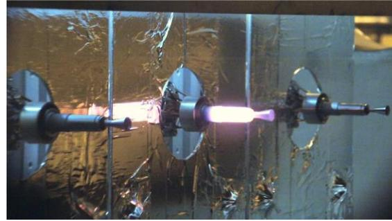
**Figure 7.** 1N HPGP thruster hot-firing in TS-2
