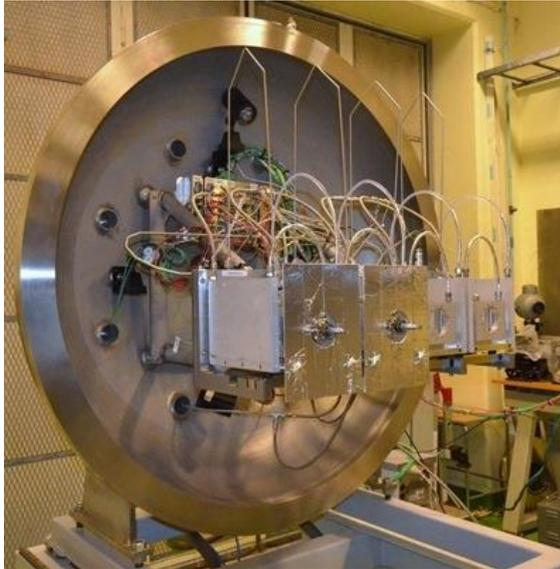
**Figure 5.** TS-2 with multiple 1N thrust balances mounted
