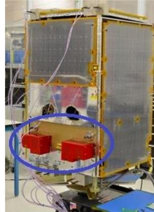
**Figure 11.** HPGP propulsion system (circled) integrated into the SkySat-3 satellite
