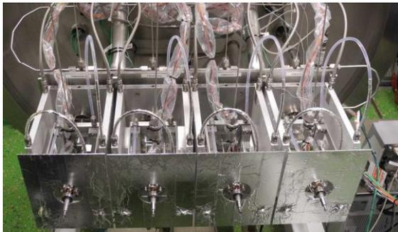
**Figure 6.** Four 1N HPGP thrusters mounted in TS-2
