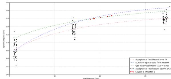
**Figure 14.** Comparison of On-Orbit Steady-State Performance vs. Pre-Flight Predictions
