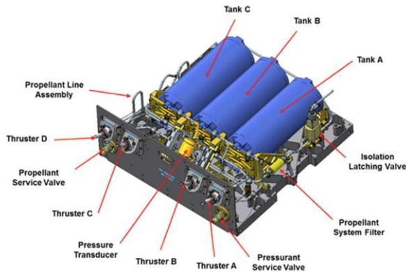
**Figure 3.** SkySat HPGP System Layout
