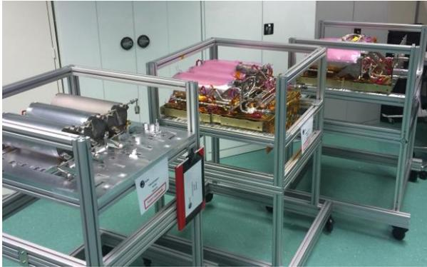
**Figure 9.** Multiple SkySat HPGP systems in different stages of production
