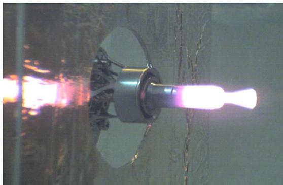
**Figure 17.** 1N GP Thruster Hot-Firing
