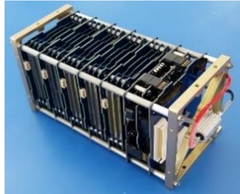
Figure 8: NewSat power subsystem batteries and power supply management unit
