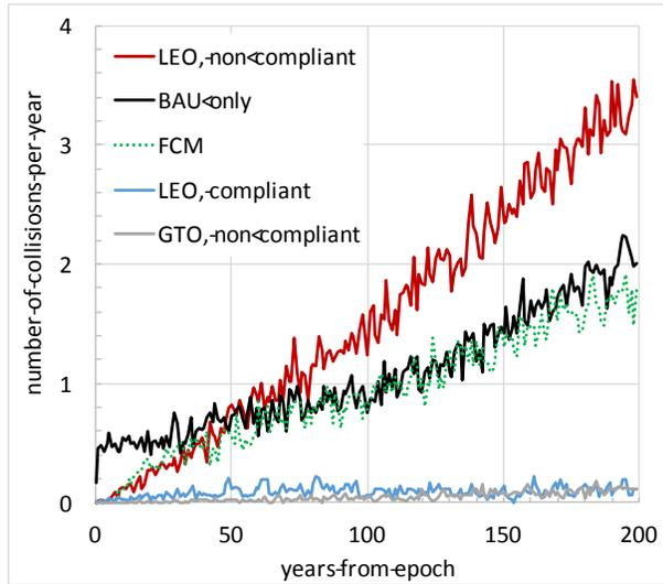
**Figure 2: Number of collisions per year for BAU-only, FCM, and CubeSat Groups averaged over 100 Monte Carlos**
