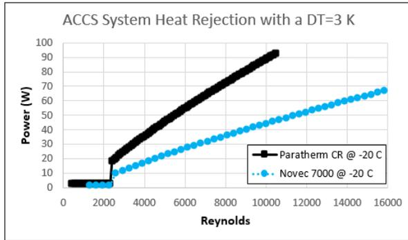
**Figure 23: ACCS System Heat Rejection vs. Reynolds for Paratherm CR & Novec 7000**
