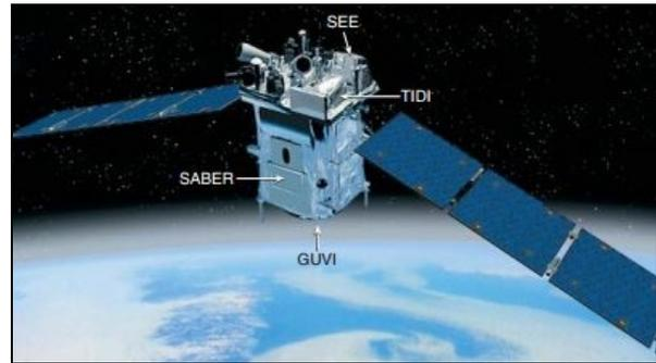
**Figure 2: Original SABER Instrument on the TIMED Spacecraft<sup>4</sup>**
