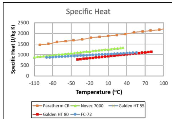
Figure 9: ACCS Working Fluid Comparison: Specific Heat
