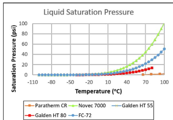
Figure 10: ACCS Working Fluid Comparison: Liquid Vapor Pressure
