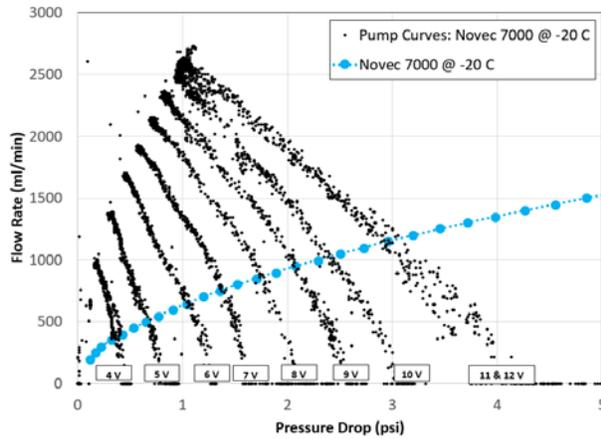
**Figure 5: ACCS System Impedance Curve Overlaid on the Measured TCS M410 Pump Characterization Curves<sup>15</sup>**
