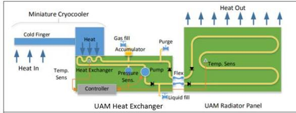
**Figure 1: ACCS MPFL Thermal Accommodation of a Cryocooler**
