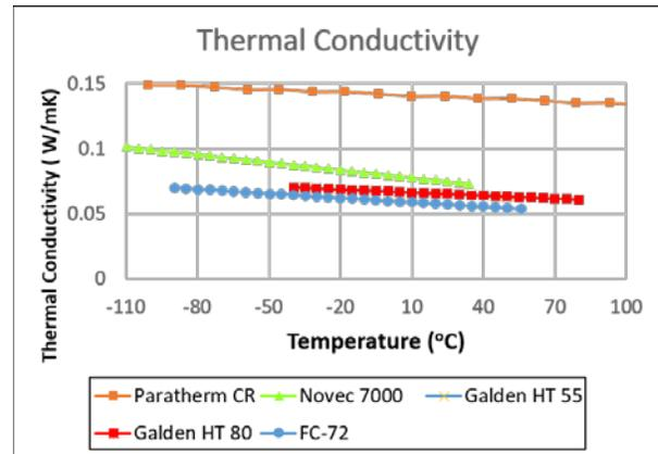
Figure 8: ACCS Working Fluid Comparison: Thermal Conductivity
