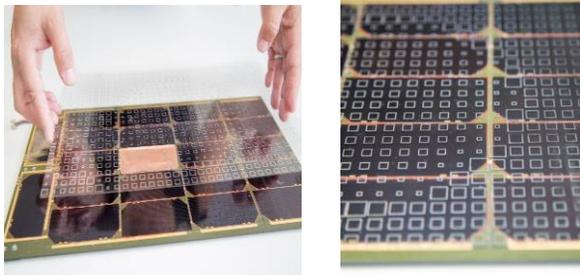
Figure 3: Antenna Placed on Solar Panel
