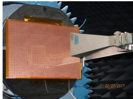
Figure 5: Close-up of Antenna under Test at Wallops
