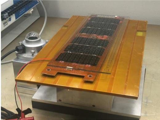
Figure 6: I-V Curve Measurement Set up
