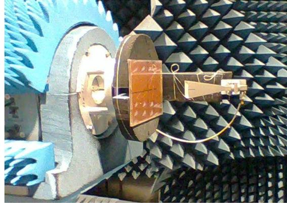
Figure 4: Antenna under Test at Wallops
