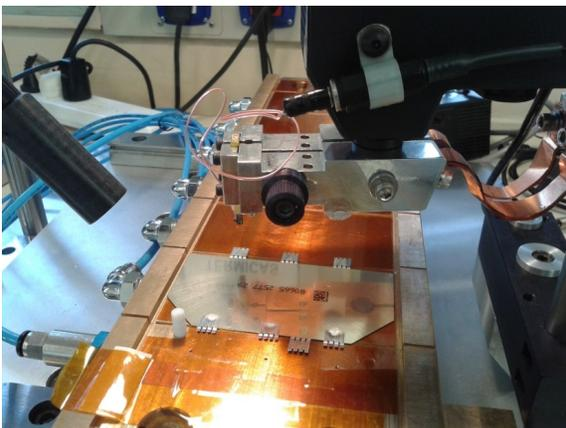
**Fig 2. Soldering process of interconnectors on the back-contact of the CIC solar cell.**
