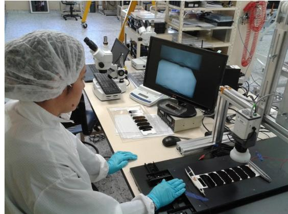
**Figure 6. Setup for mechanical inspection of cells trough E.L. The camera caps the light emitted by the GaAs subcell (about 800nm) and the image is evaluated with a good detail in the monitor.**
