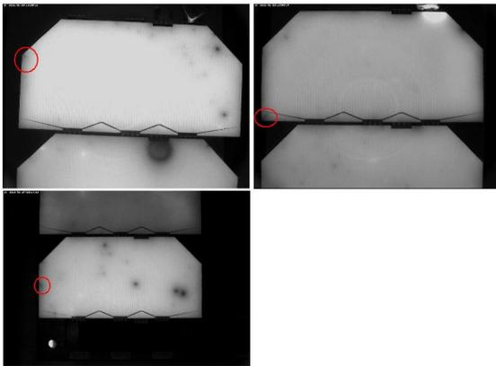
**Fig 5. Small crackings at the cells are detected trough E.L. technique. The size of the cracks in these cases presented not represents a risk for the solar module**
