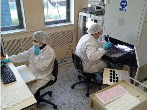
**Figure 1: Measurement of the I-V curve of individual CIC solar cell under standard test conditions are performed using a close match AM0 solar simulator.**
