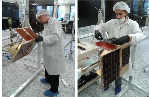
**Fig 3. Cabling and string cell bounding process are shown**
