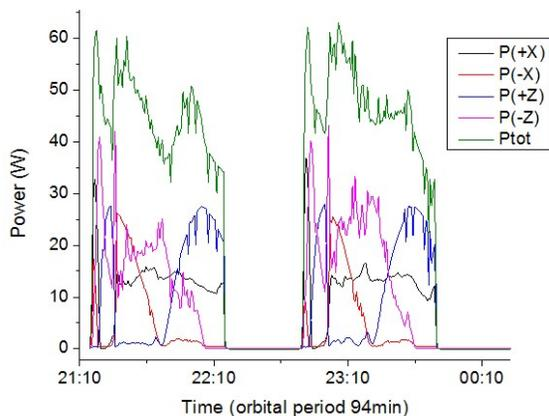
**Fig 10. Solar panels power profile during two consecutive periods from in-flight data telemetry**
