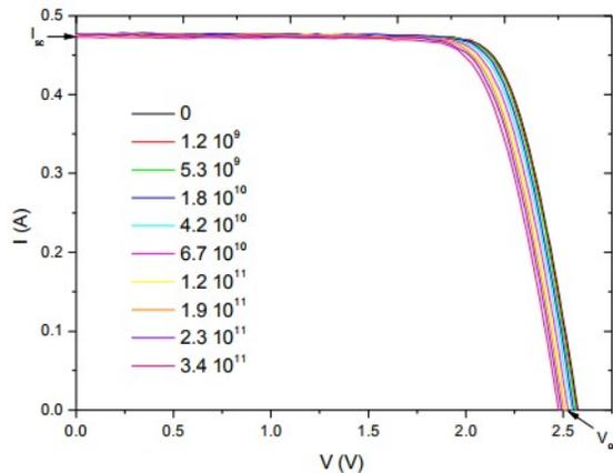
**Fig 8. I-V curves of a commercial triple junction cell measured in-situ during a radiation damage test. The fluences specified are in protons/cm<sup>2</sup>**
