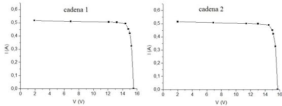
**Figure 4. Typical IV curve of six-cell string using multi-flash method.**
