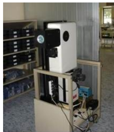
Figure 8. Simple solar simulator based on a 1 kW Xe.
