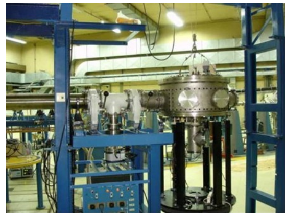
Figure 10: 76-cm vacuum chamber installed on one of the Tandem accelerator beam lines.
