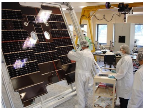
Figure 5. Substrings of cells are bonded to the SAC-D substrate.
