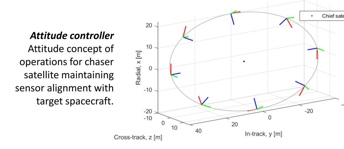
Model predictive control is used for closed-loop control during close-proximity operations and docking with the apogee engine. *Multi-objective cost function* to allow for greater control over
