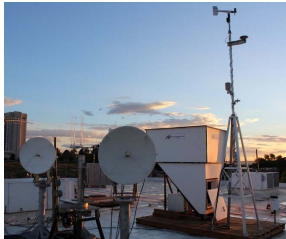
Figure 2 WTLE 72 GHz and 82 GHz Test Experiment on the COSMIAC Roof
