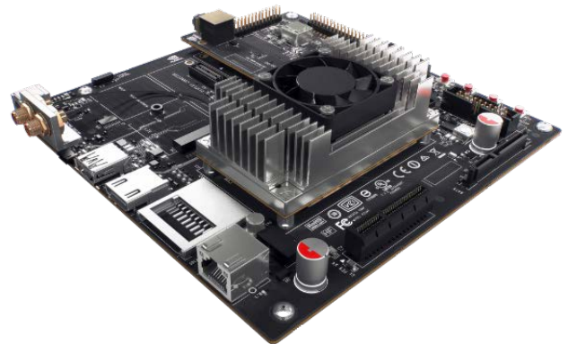
Figure 2: Jetson TX1 development board; the silver heatsink with black fan covers the TX1 SoC module. 5
