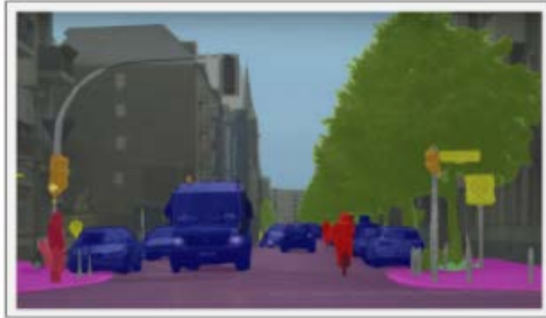
Figure 5: Example of image segmentation with segNet; this example model identifies and separates a multitude of different object types in an urban setting. 3
