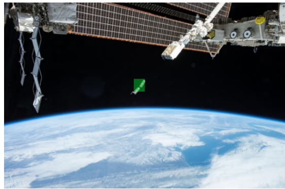
Figure 15: Two 3U-sized CubeSats just after NanoRacks deployment from the International Space Station (ISS). Notice at greater distance the model does not distinguish two separate objects; photo credit: NanoRacks.
