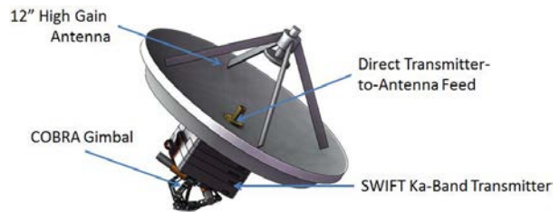
Figure 11: COBRA Gimbal with SWIFT Ka-band Transmitter and High Gain Antenna
