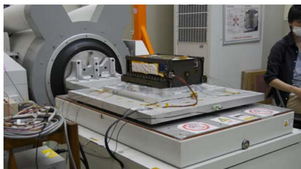
Figure 17: Configuration of EQUULEUS vibration test
