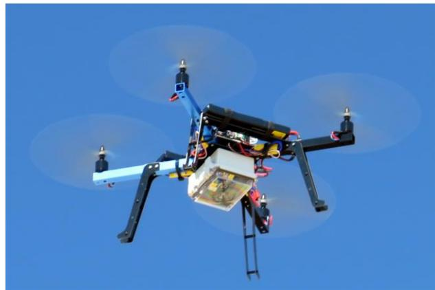
**Figure 8. Quadcopter Test Vehicle with Mesh Network Payload**
