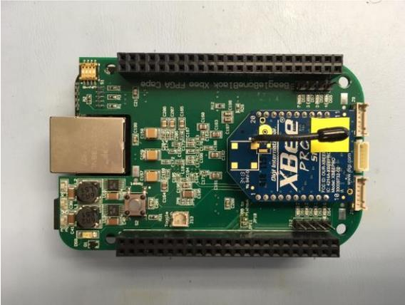
**Figure 6. Third Generation XBee Node Stack**
