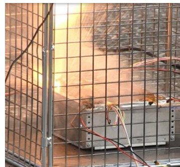
Figure 13. Test Battery induced into thermal runaway
