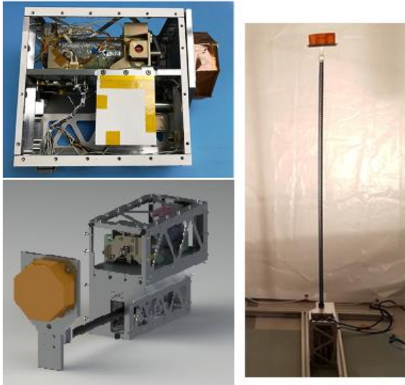
Figure 8. Top Left: inside the Harpoon target assembly (HTA); Bottom Left: CAD model of HTA with target partially deployed. Right: HTA with CPRF boom fully deployed during fire testing (HTA at bottom, target plate at top).
