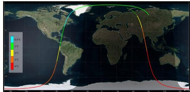
**Figure 12: HyperScout® telescope temperature variations through out the commissioning orbit.**
