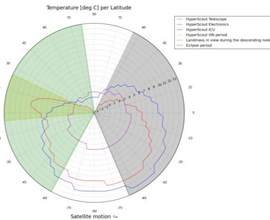
**Figure 11: HyperScout® subsystems temperature plot relative to the revolution of the Cuba acquisition**
