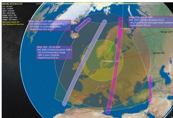
**Figure 6: HyperScout® operations for the acquisition of the first commissioning image.**
