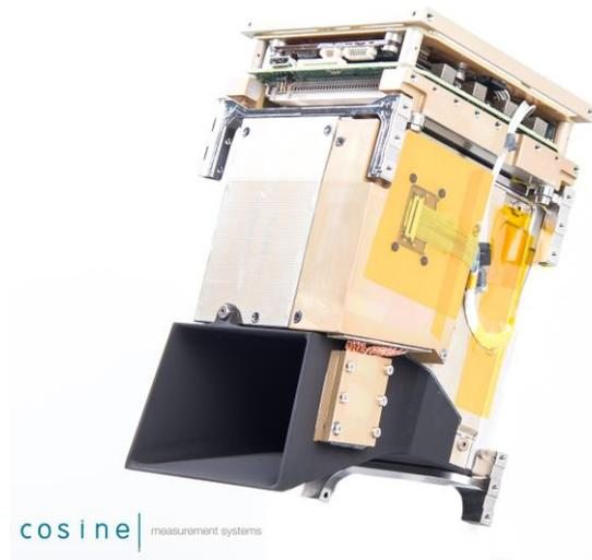
**Figure 1: HyperScout Flight Model**
