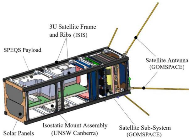
**Figure 2: SpooQySat layout with interstage panels, side solar panels, harnesses removed<sup>19</sup>**
