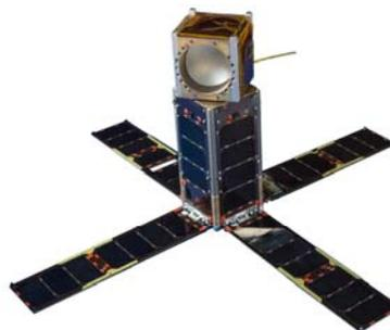
**Figure 1: The MicroMAS-2a satellite is 4.5 kg and 34 x 10 x 10 cm<sup>3</sup>**
