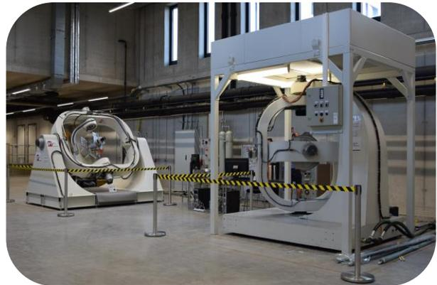
**Figure 6: Dynamic Bench Test Facility at ZfT premises for three-axis satellite motion simulation**
