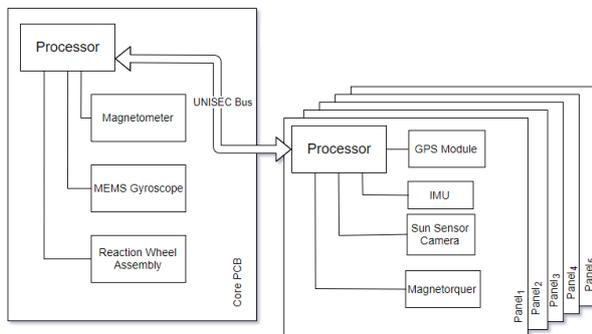
**Figure 4: Distributed functionalities of the QUBE ADCS<sup>2</sup>**
