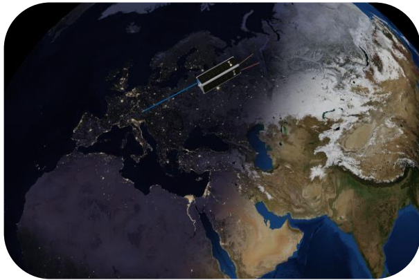
Figure 8: QUBE orbit simulation with optical laser link during eclipse
