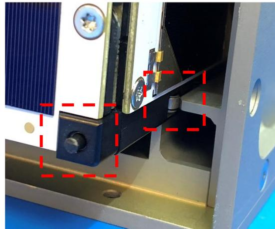
**Figure 1: Deployment Switch Configurations**
