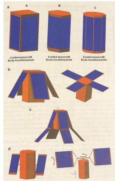
**Figure 3: Example Body-mounted Arrays<sup>12</sup>**
