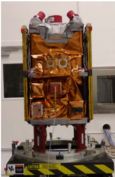
Figure 6: GPIM Space Vehicle. The GPIM mission leverages a flight heritage BCP-100 Spacecraft and a flight demonstration AF-M315E propellant propulsion subsystem.
