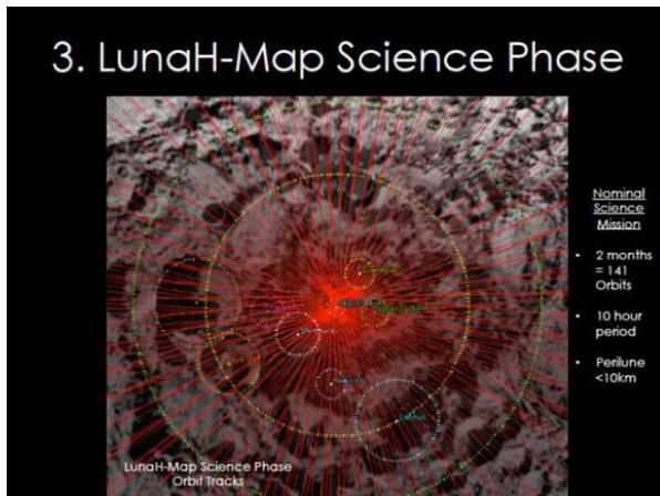
**Figure 6: LunaH-Map Science Measurement Coverage for South Pole**
