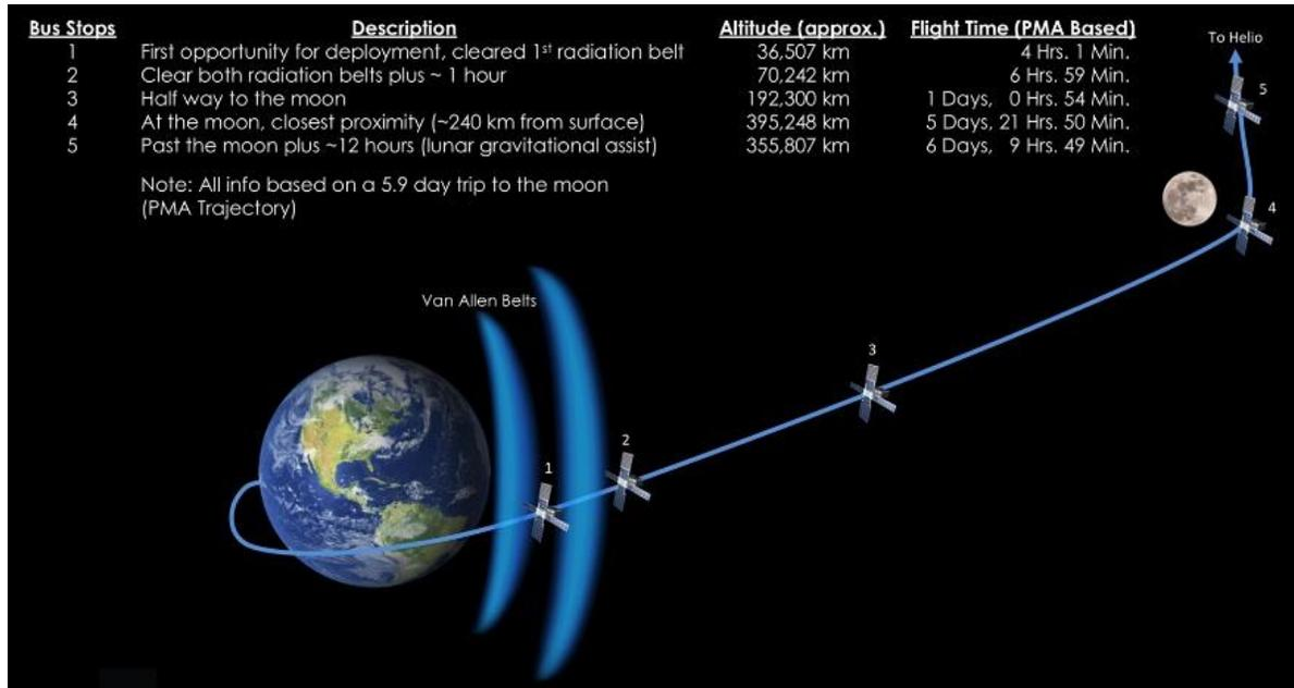
**Figure 4. Providing smallsats with extraordinary access to deep space, SLS presented payload developers with several “bus stops,” or deployment opportunities, for the first mission; similar opportunities are expected to be available on future missions.**
