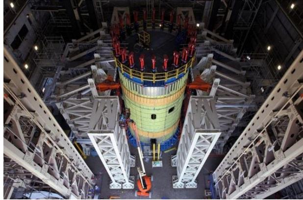
**Figure 12. The next core stage component to undergo structural testing is the intertank structural test article, consisting of a full-size replica of the intertank and simulators for the liquid oxygen and liquid hydrogen tanks.**
