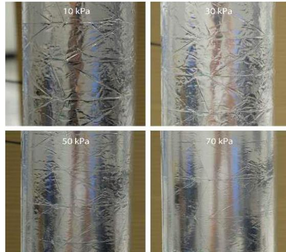
**Figure 4. Residual Creases after Depressurisation from Different Inflation Pressures (10–70 kPa)**
