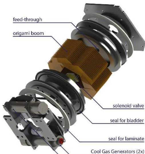
**Figure 8. Inflatable Mast (Boom) System Layout**
