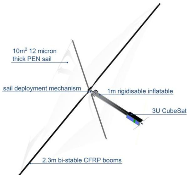
**Figure 3. Artist's Impression of InflateSail in Orbit Deployed Configuration Showing the 1m Long Inflatable Cylindrical Mast and the 10m<sup>2</sup> Drag Augmentation Sail Supported by 4 CFRP Booms**
