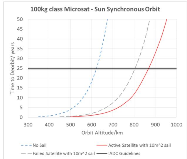
**Figure 23. Performance of a 10m<sup>2</sup> dragsail mounted to a 100kg microsat**
