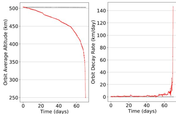
**Figure 19. InflateSail’s Changes in Altitude and Decay Rate**
