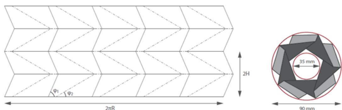
**Figure 6. The Fold Pattern Selected for the Inflatable Mast (left), with the Cross-Sectional View of its Fully Folded Configuration (right). The fold pattern is fully defined by its geometric parameters  $n = 5$ ,  $\phi_1 = 67^\circ$ ,  $H/R = 0.67$  and  $R = 45\text{mm}$ . In its fully stowed configuration the diameter of the circumscribed circle is 90 mm, and the open cross-section is at least 35 mm in diameter.**
