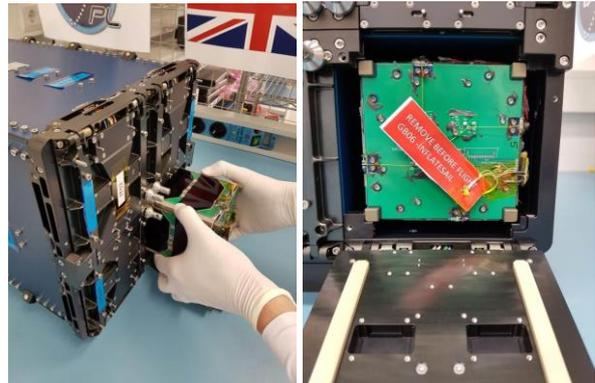
**Figure 15. InflateSail Being Integrated into the ISIS QuadPack**
