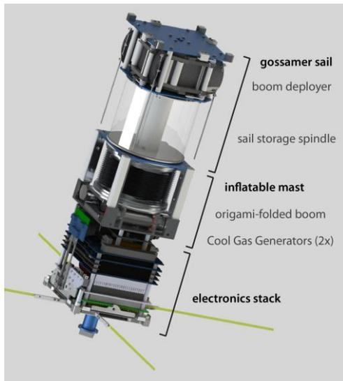
**Figure 2. CAD Representation of InflateSail's Internal Layout**
