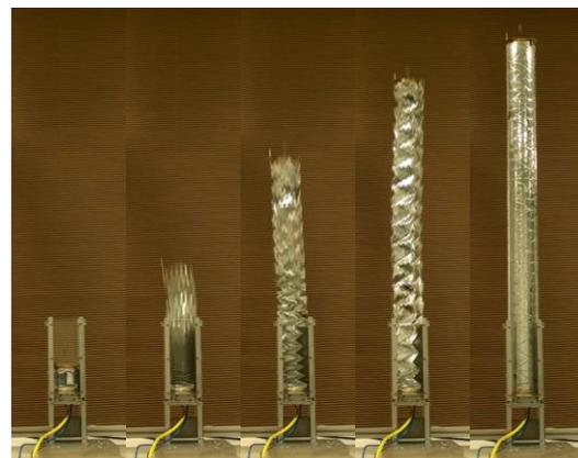
**Figure 5. The Inflatable Cylindrical Mast Deployment Sequence**
