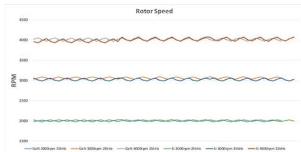
Figure 6: Speed Ripple GaN versus Si (at 25kHz)
