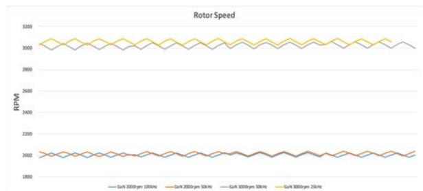
Figure 7: Speed Ripple GaN (25kHz vs 100kHz)
