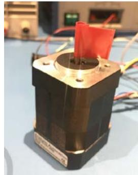
Figure 2: BLDC motor illustration
