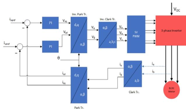
Figure 1: Basic Scheme of FOC
