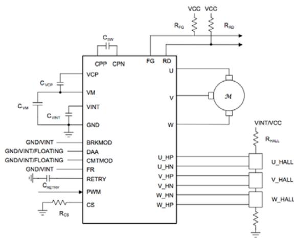
Figure 4: Electric Schematics of the Si Drive<sup>10</sup>
