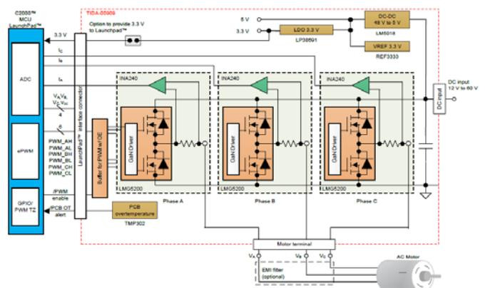
Figure 3: Schematics of GaN motor drive module<sup>3</sup>
