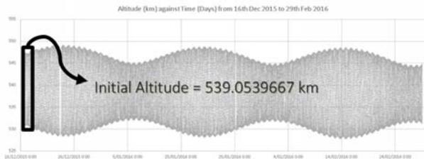
Fig 3: Actual GPS data for VELOX-CI satellite on 16/12/2015
