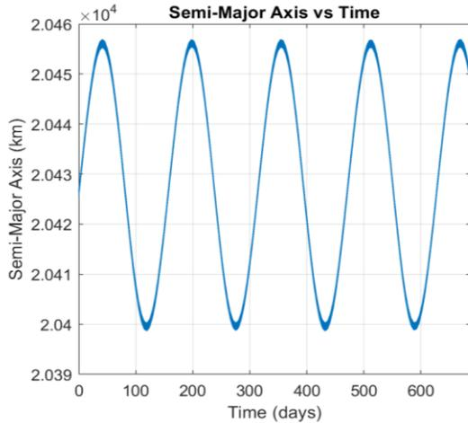
**Figure 3. Semi-Major Axis oscillating over a one year time span due to the Spherical Harmonics of Mars caused by mountainous regions and crustal variations.**
