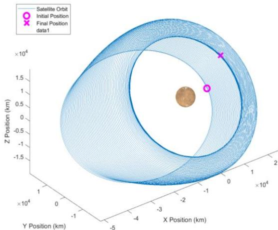
**Figure 4. Controlled Transfer from high to zero eccentricity**
