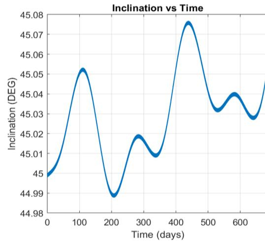
**Figure 3. Inclination changes over a one year time span caused by a number of factors including the moons, Phobos and Deimos, and the sun.**
