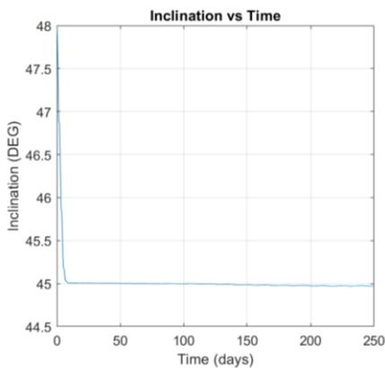
**Figure 7. Inclination targeting of 45 degrees for Example transfer.**
