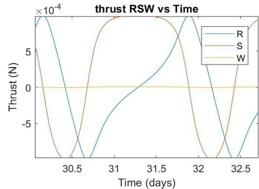
**Figure 8. Thrust components produce by electric thruster for the controlled example simulation**
