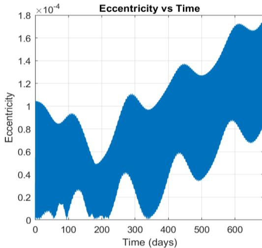
**Figure 3. Small eccentricity variations increasing slowly over time mostly due to Solar gravity acting on the satellite.**
