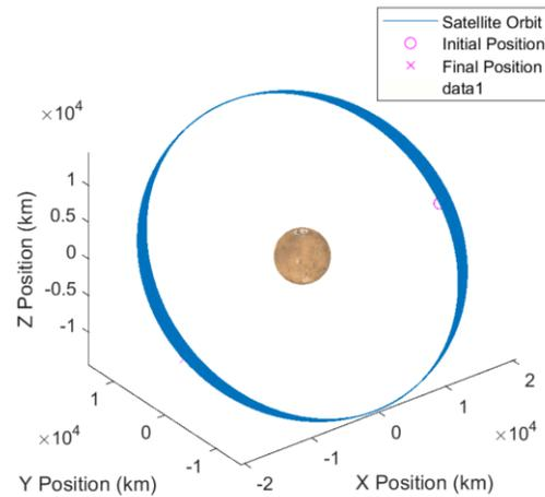
Figure 2. Coasting Orbit around Mars.
