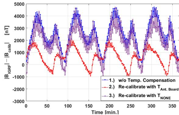
**Figure 6: Test with New Runs of In-Flight Data: Magnitude Errors of Calibration with 1.) Only Bias, Scale Factors and Misalignment terms. 2.) All Calibrated Parameters and  $T_{\text{Ant. Board}}$ . 3.) Parameters from Comparison Test ( $T_{\text{NONE}}$ ).**
