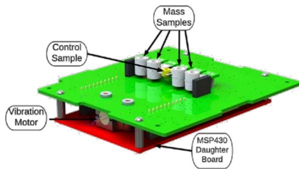
Fig 11. Drawing of the polymer mass loss experiment
