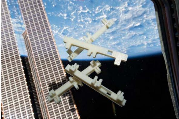
Fig 1. MakerSat-1 frame 3D printed onboard the ISS
