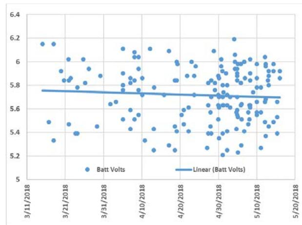
Fig 6b. Battery Voltage vs. Time (solar-locked state)
