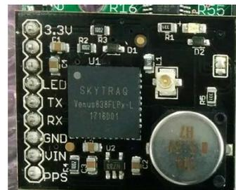
**Figure 4: GPS module used in BIRDS-2 project**
