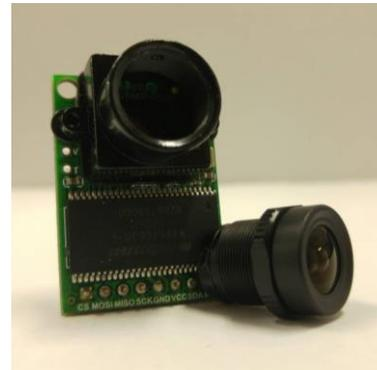
**Figure 3: Camera module used in BIRDS-2 project**
