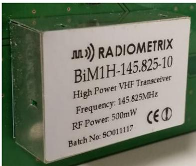
**Figure 2: VHF transceiver payload of BIRDS-2 project**
