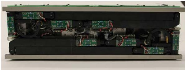
**Figure 2: RSat Robotic Arm**
