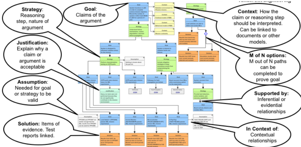
Figure 6. Explanation of Goal Structuring notation [2]
