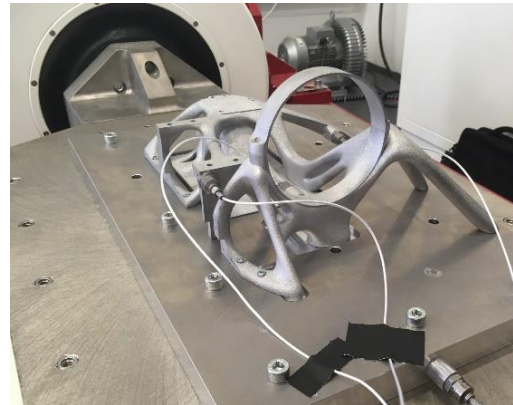
Figure 9: Optical bench shaker setup
