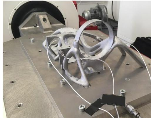
**Figure 9: Optical bench shaker setup**
