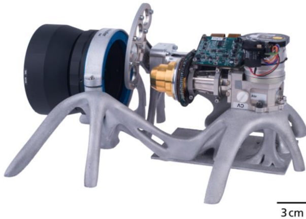
Figure 8: Additive manufactured optical bench
