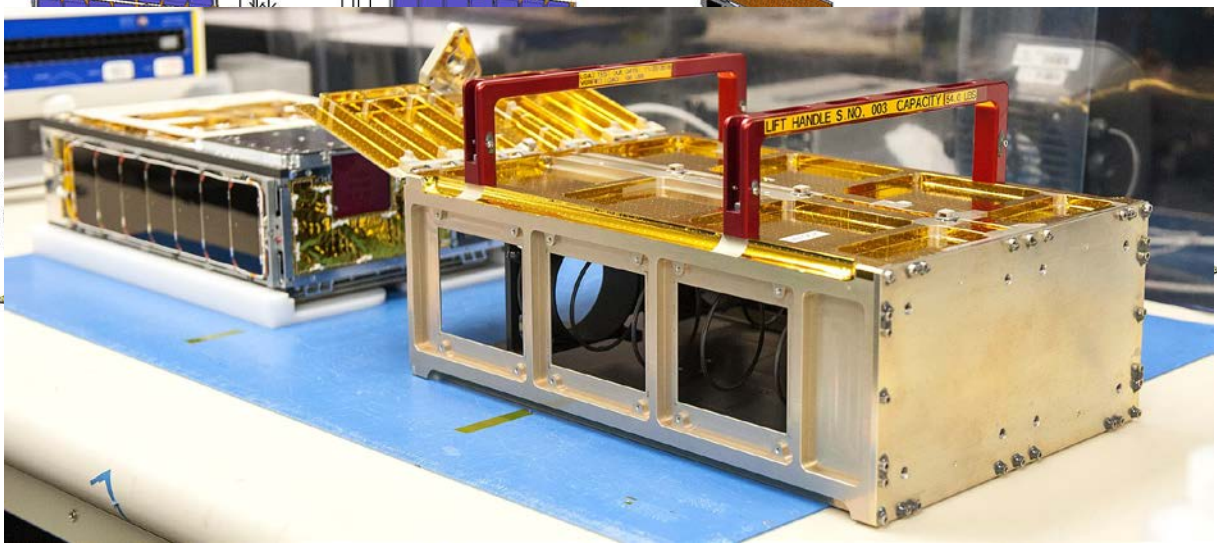
Figure 1: Schematic of the Mars Cube One spacecraft (front and back) with front panel removed.
