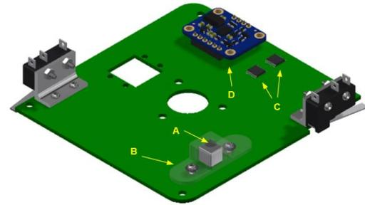
**Figure 6: The ADCS circuit board. A - neodymium magnet. B - magnet's flange. C - analog to digital converters. D - IMU.**
