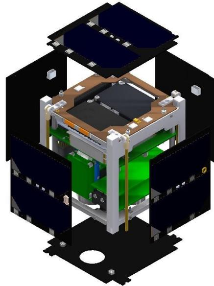
**Figure 3: Arrangement of the components to the structure.**
