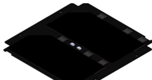
Figure 8: Location of the two photodiodes in every CubeSat's face.
