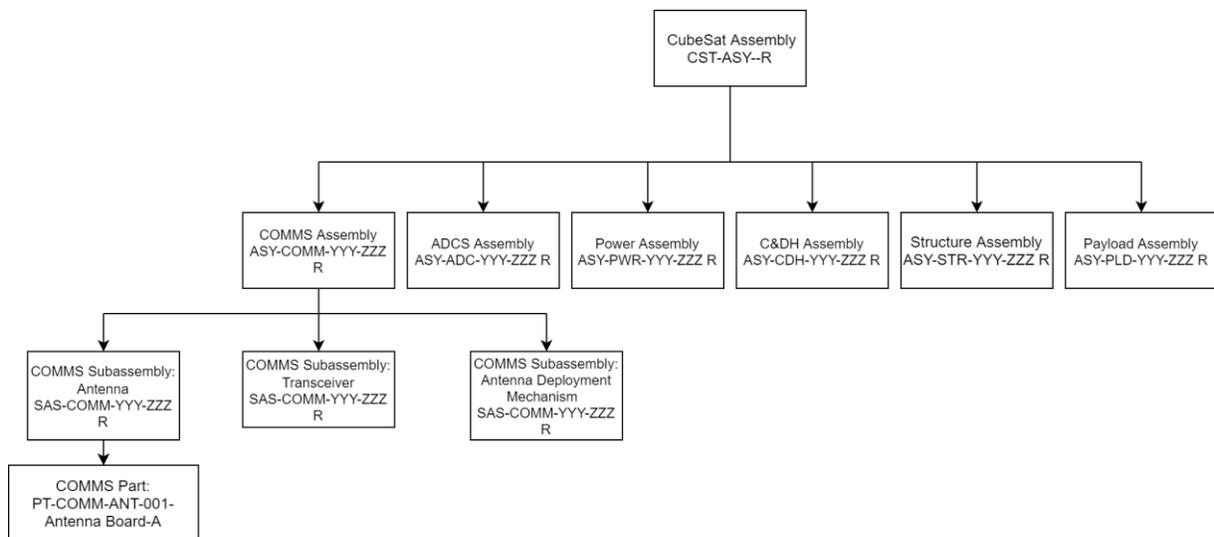
**Figure 10: Engineering drawing organization tree, designed to convey the hierarchical structure of each drawing in the engineer drawing package. Starting from the main assembly, the submodules, the subassemblies and specific parts.**
