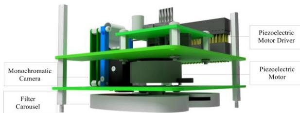
**Figure 1: Payload components arrangement.**
