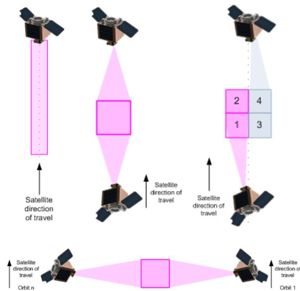
**Figure 9: Carbonite-2 imaging modes**
