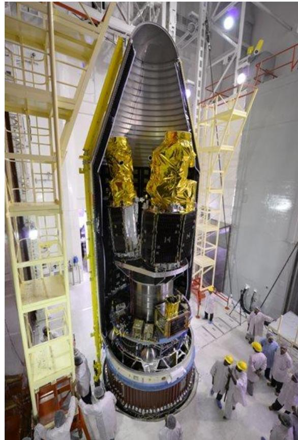
**Figure 4: DMC3 and Carbonite-1 satellites in shared PSLV-XL launch**
