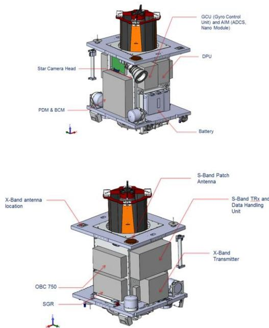
**Figure 7: Carbonite-2 configuration**
