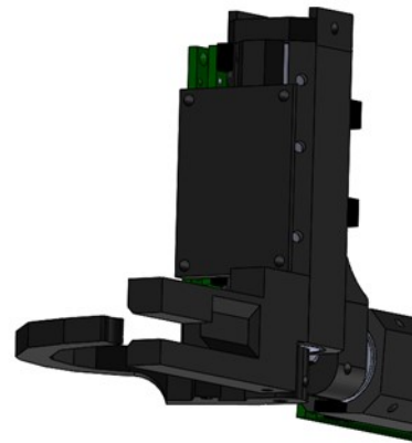
Figure 7: ISAR End Effector “Claw” Design
