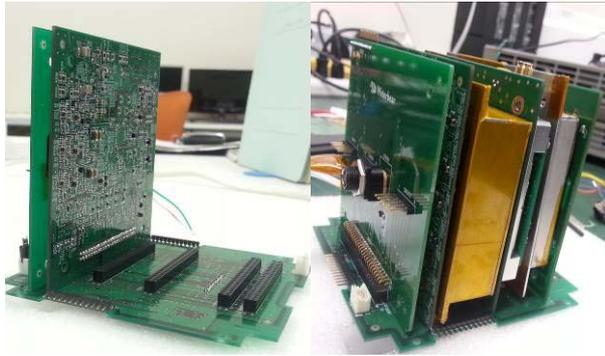
**Figure 1. An example of the backplane board for 1U CubeSats with subsystems**
