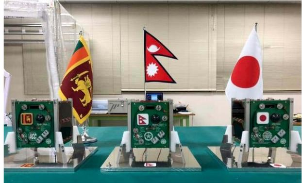
**Figure 4. Flight models of the BIRDS-3 CubeSats**
