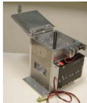
**Figure 3: CubeSat XI-IV's separation mechanism**
