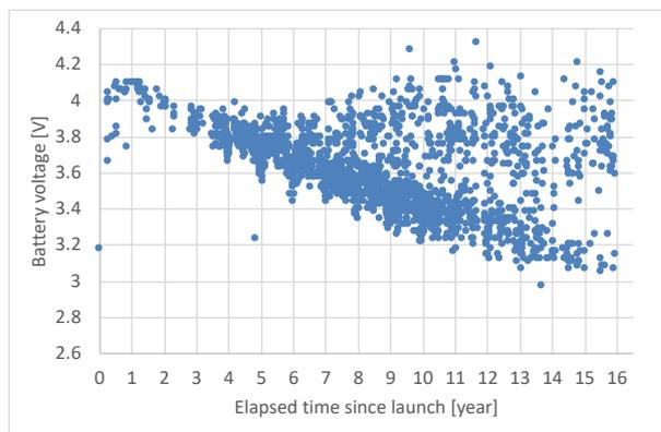
**Figure 5: 15-years trend of battery voltage**
