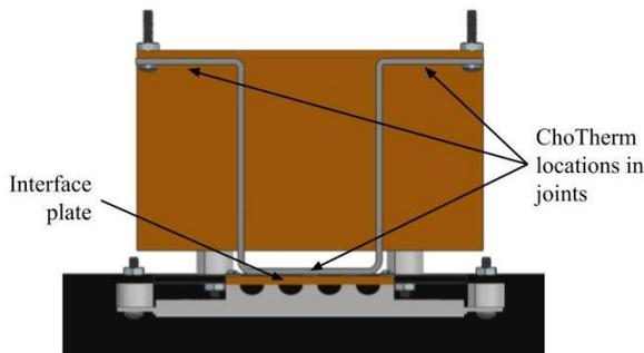
**Figure 3: CAD model side view of copper ribbon.**
