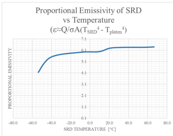
As this graph shows, the emissivity of the SRDs is increasing with temperature. Future analyses using simulations with a thermal math model will enable higher accuracy in the value of  $Q$  to use in Equation (1) in order to provide better emissivity estimates.
