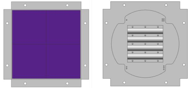
**Figure 1: CAD model of SRD plate- SRD mounting side on left, heat pipe interface side on right.**
