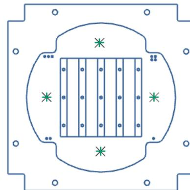
**Figure 5: Location of thermistors on heat pipe-interface side of SRD plate.**
