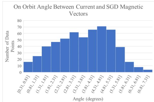
**Figure 11: A histogram of the on-orbit angular difference between existing and SGD magnetic vectors**
