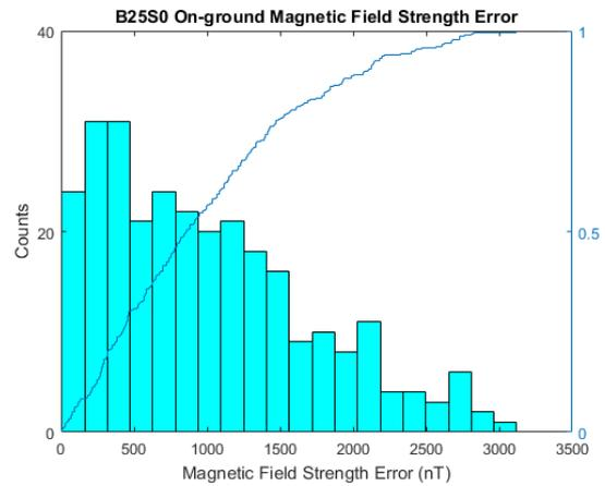
**Figure 5: On-ground B1SB calibration values magnetic field strength error**
