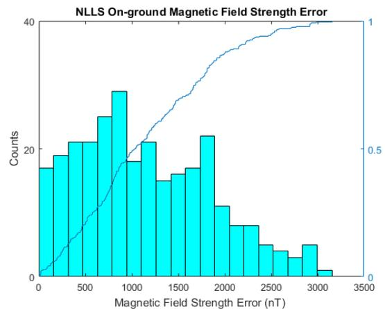
**Figure 6: On-ground B25S0 calibration values magnetic field strength error**
