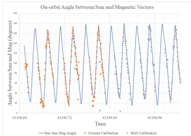
**Figure 8: On-orbit measured angle between sun and magnetic vector comparison**
