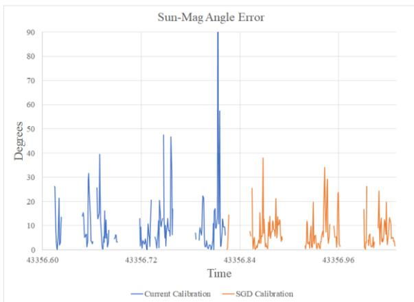
**Figure 10: On-orbit angle between sun and magnetic vector error comparison**
