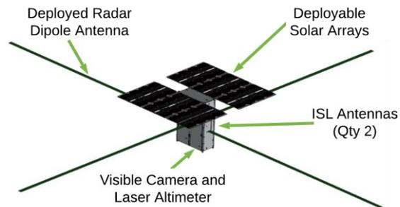
**Figure 5: Juventas in the Deployed Configuration**
