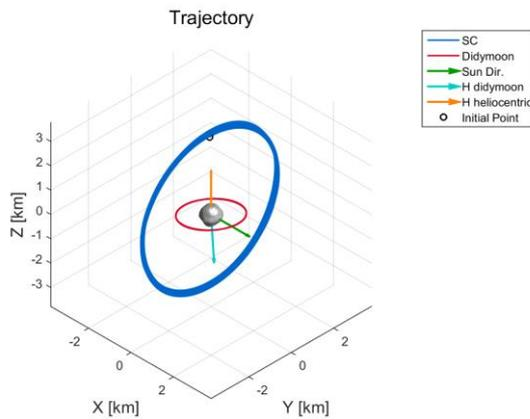
**Figure 2: Juventas Self-Stabilizing Terminator Orbit (SSTO) around Didymos**
