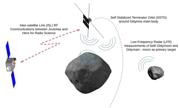
**Figure 3: Juventas Observation Phase for Radar and Radio Science**
