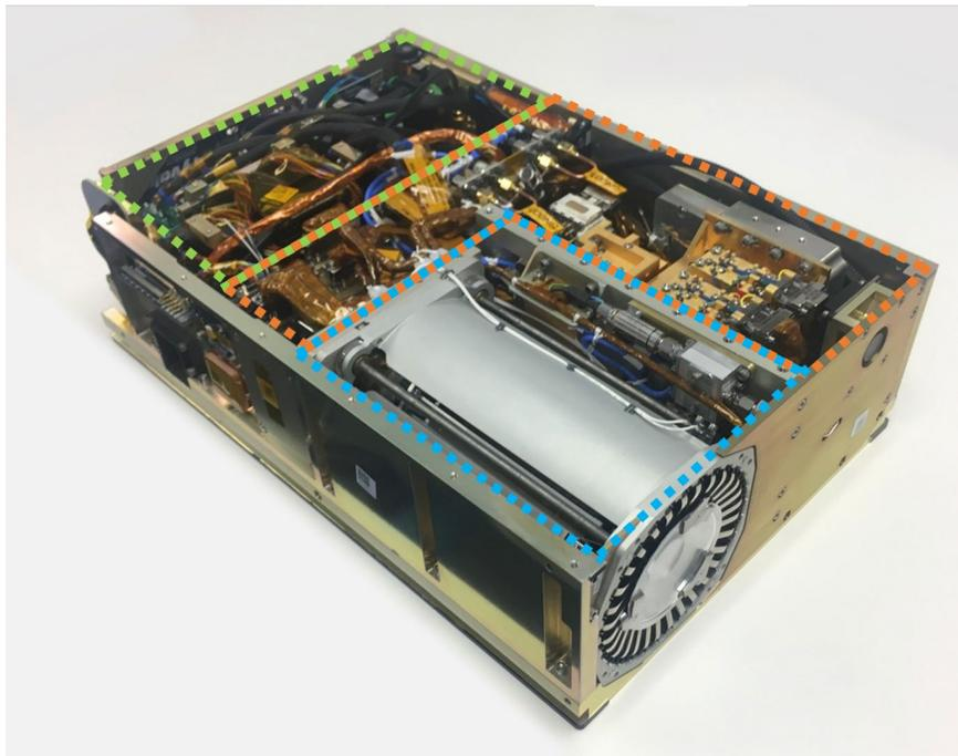
**Figure 2. The mini-KaARC radar electronics (orange line), KARPDA deployable antenna (blue line), and spacecraft bus (green line), integrated into the flight chassis, prior to launch**
