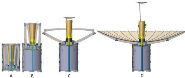
**Figure 3: The deployment sequence unfurls the 0.5m antenna from a 0.1m diameter cylinder.**
