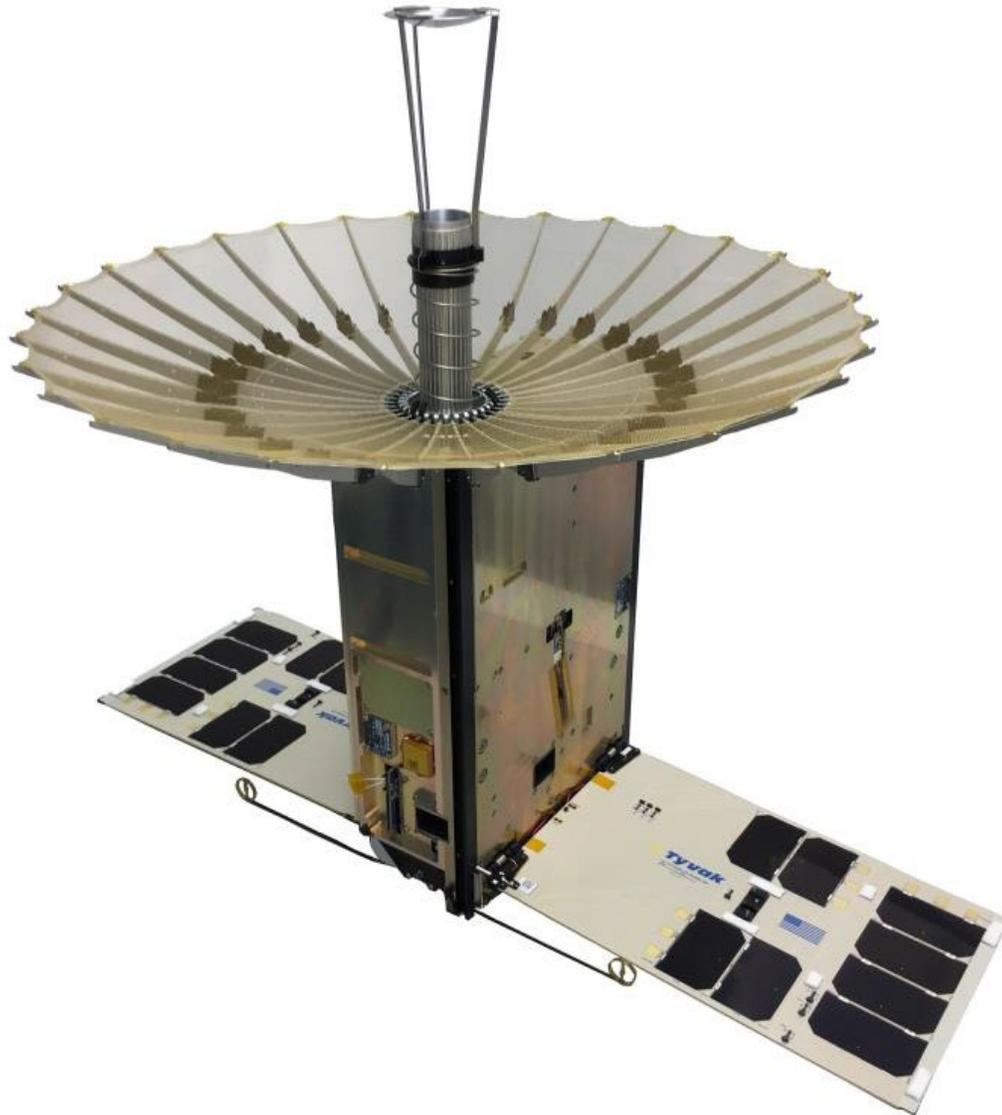
**Figure 1. The RainCube 6U CubeSat fits the 0.5m antenna into 1.5U, the radar electronics into 1.5U, and the spacecraft bus into 2U. The vehicle has deployable solar panels and UHF antennas.**
