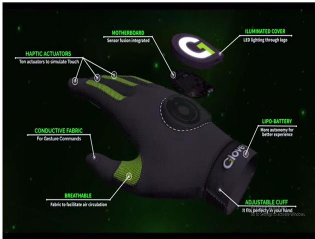
**Figure 9: Haptic Actuator Example**
