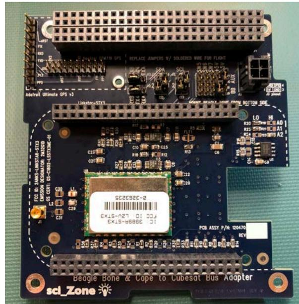
**Figure 6: The LinkStar-STX3-PC104 Radio System.**
