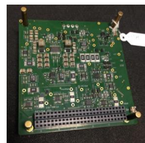
Figure 6: Eye-Sat's power board
