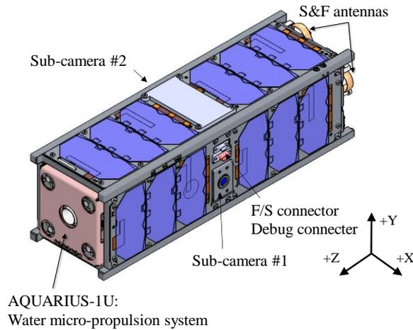
**Figure 1: CAD model of AQT-D spacecraft**
