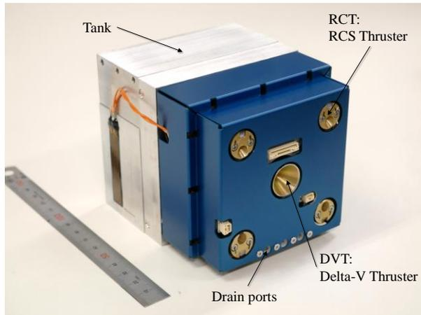
**Figure 4: Photograph of the water micro-propulsion system**
