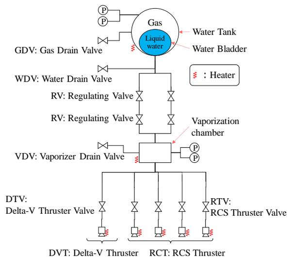
**Figure 3: System diagram of the water micro-propulsion system**
