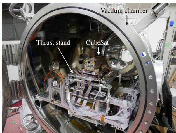
**Figure 8: Experimental setup of the integrated firing test. Thrust profile during the firing was directly measured by using the thrust stand.**
