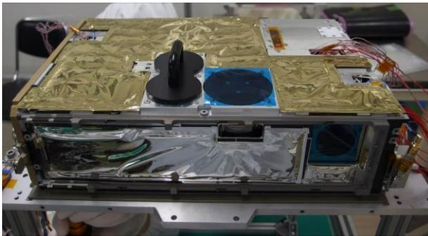
**Figure 12: Flight model of EQUULEUS w/o SAP**
